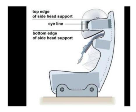
If a foam insert is used between the homologated seat and the driver, minimum lateral support to the driver's head, shoulders and pelvis must be quaranteed as follows:
